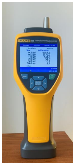
Figure 1: The particle counter, measuring the number of particles per liter of air of a given size indicated in the display. When aerosols are produced, these are visible as an increase in the different channels over the background (dust) particles. The average size of aerosols produced by human activity is around 5 \mu\text{m} [9], after evaporation of the water contained in saliva this gives rise to aerosols of about 1-2 \mu\text{m} . We thus use this size range also for the production of the artificial aerosols; the measurements presented below show the data for the 1 \mu\text{m} channel, however other channels give similar results and especially the same persistence time to within the experimental accuracy.
