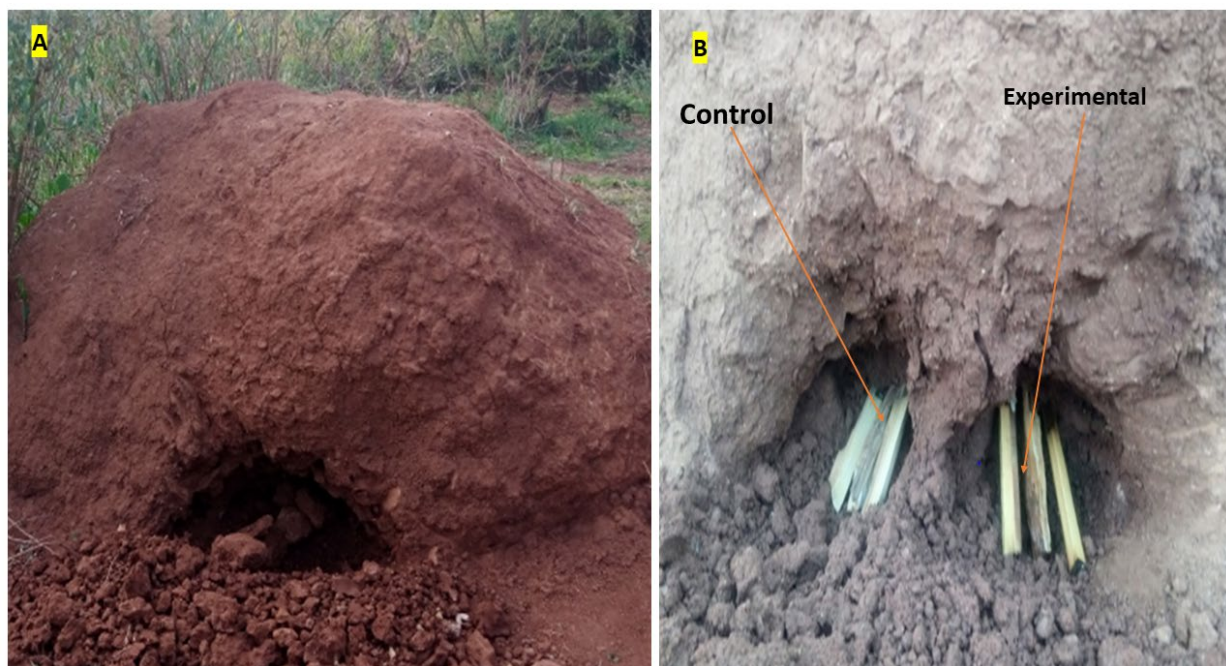
Figure 1. Excavated mound (a), control and experimental wood samples placed in the mound (b).
